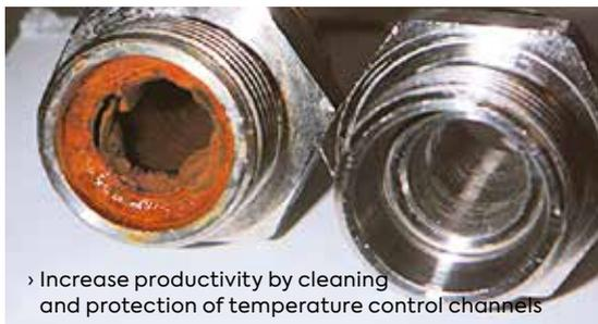
› Increase productivity by cleaning and protection of temperature control channels
