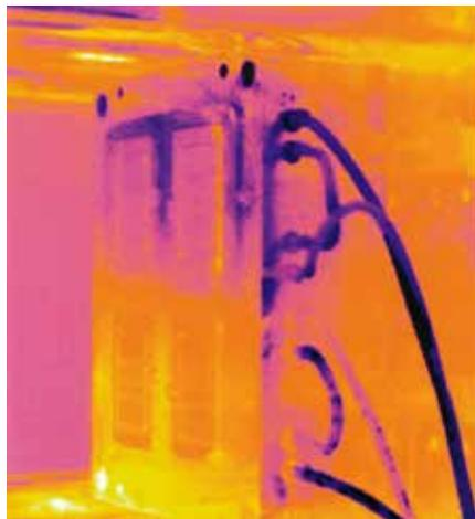
› Inhomogeneous temperature distribution in the injection mould due to polluted temperature conditioning circuits.
