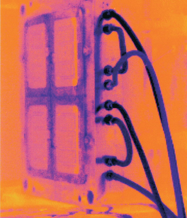
› Homogeneous temperature distribution after flushing the mould and conditioning the water
