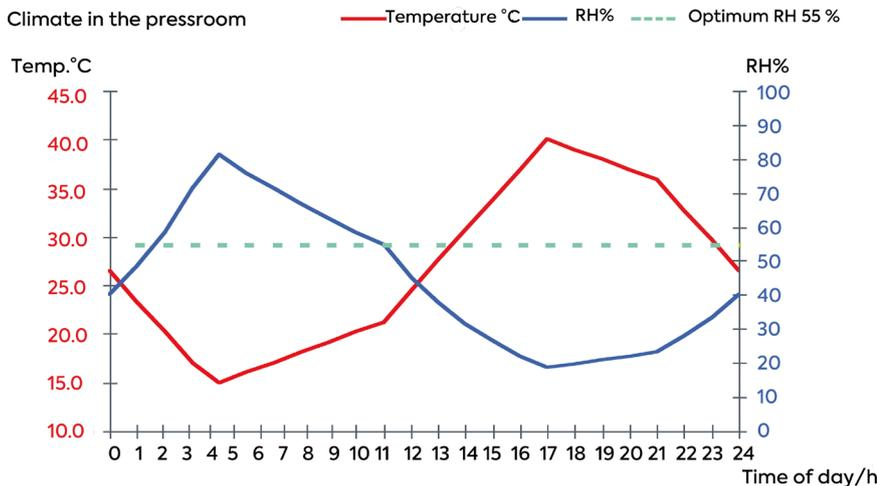
› The relative humidity of an area is directly dependent on the air temperature. The physical law shown here is quite simple: rising air temperature leads to decreasing relative humidity and vice versa. Fluctuating ambient conditions have a notable negative impact on the printing papers.
