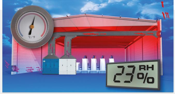
› By adding waste air ventilation and exhaust ducting, the heat can be removed but the extra air needed for pressurisation permanently disturbs the climate of the printing room.
