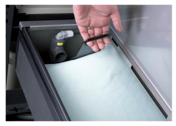
The filter bag cleans effectively in tank: softflow – up to 300 % larger filter area compared to filter mat.
